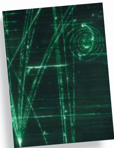
Figure 2.32 High-energy subatomic particles leave telltale tracks in an experimental cloud chamber.
