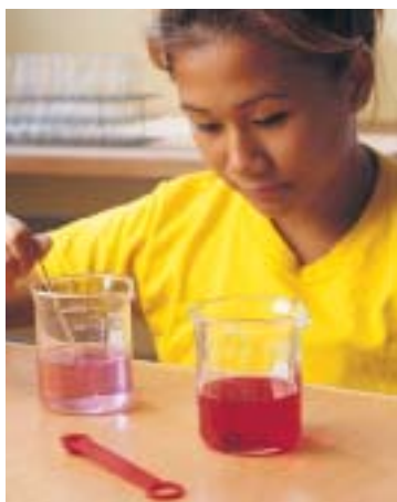
Figure 2.3 The beaker above has 1 part food colouring for every 100 parts of solution. The other beaker below has 100 ppm.
