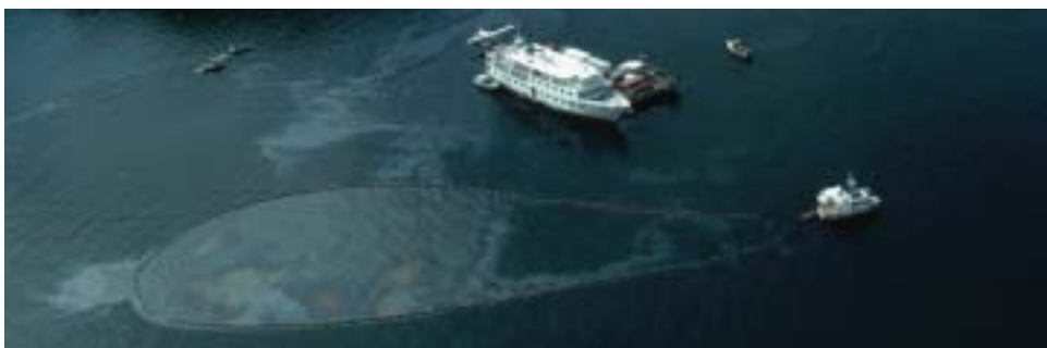
Figure 3.16 Booms can be used to contain oil spills and help with clean-up.
